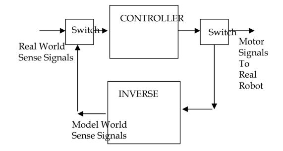
**Normal Mode** – controller produces motor signals, inverse detects mismatch or *novelty*.
